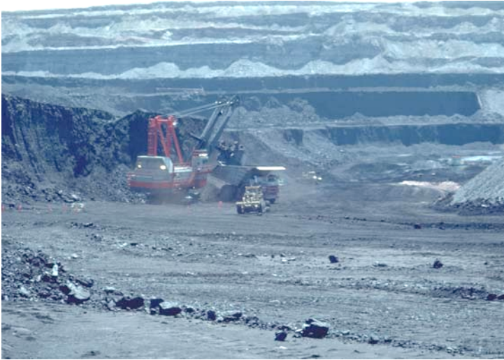
Figure 6. Electric shovel loading truck in strip mine. 20
